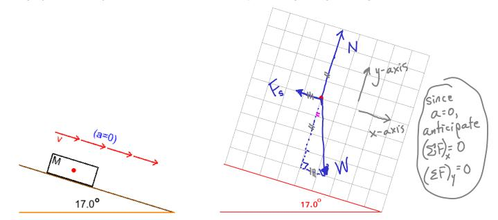
/1 (1.a) In the grid space above right, construct a free body diagram (or force diagram) for the sliding mass. This should also include a coordinate system.
