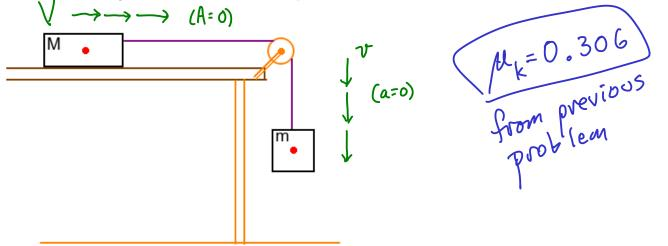
(2.a) Construct free body diagrams (or force diagrams) for the sliding mass and the hanging mass. This should also include a coordinate system. Your diagrams should also include coordinate axes. (You should also make motion diagrams.)
