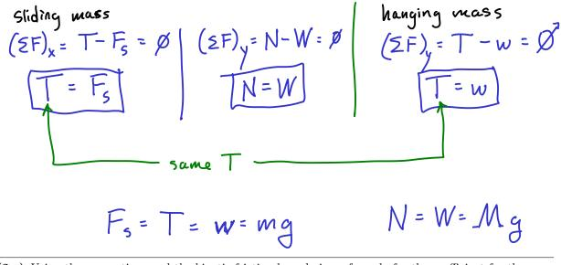
/2 (2.c) Using those equations and the kinetic friction law, derive a formula for the coefficient for the hanging mass m in terms other measured or given quantities.
